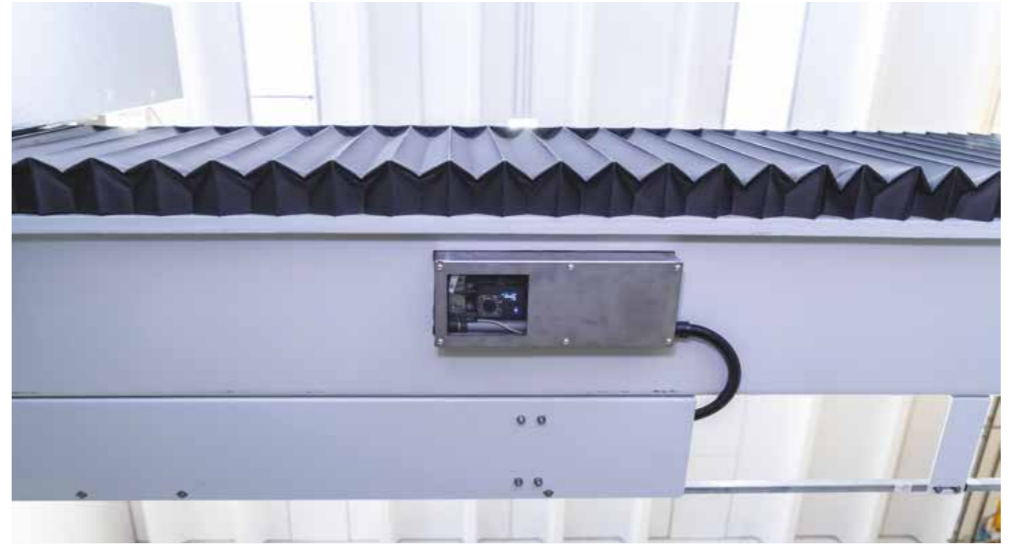
CAMERA: system to obtain the images from the working table, it permits to accelerate the pieces positioning and notice possible bugs on the slab
