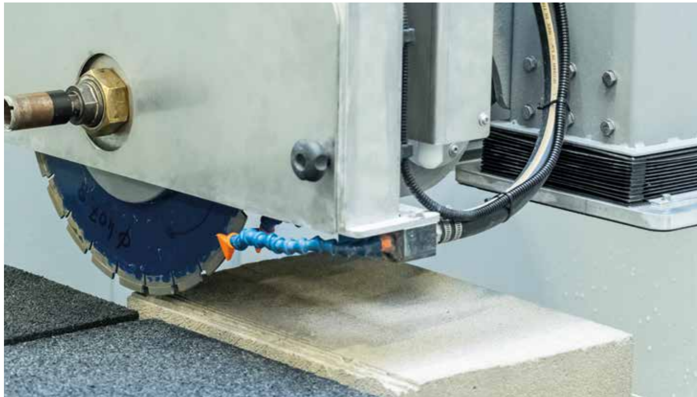
DISCK AUTOMATIC RESTART STATION it can be activated by a specific funtion on the operator panel
