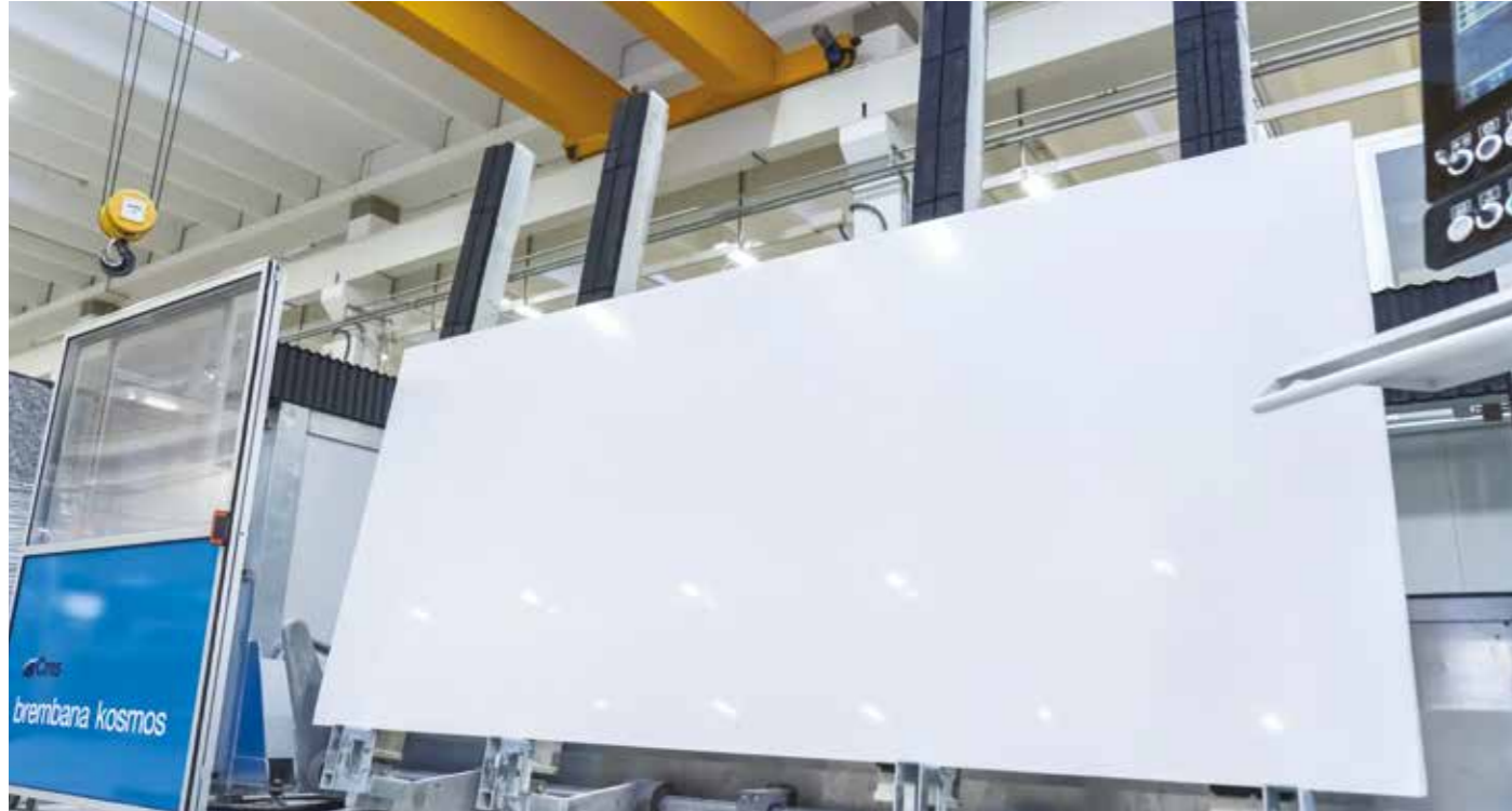
WORKBENCH with four flap forks (optional, with a maximum capacity of up to 800 kg) and dimensions of 4,000 x 2,350 mm; the work table is in rectified rubber
