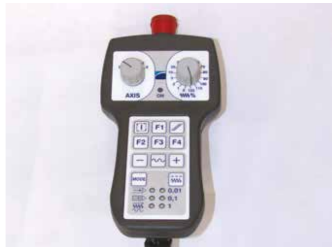
Remote control unit for driving up to 6 axes; it allows you to operate close to the cutting table and set multiple starting points.
