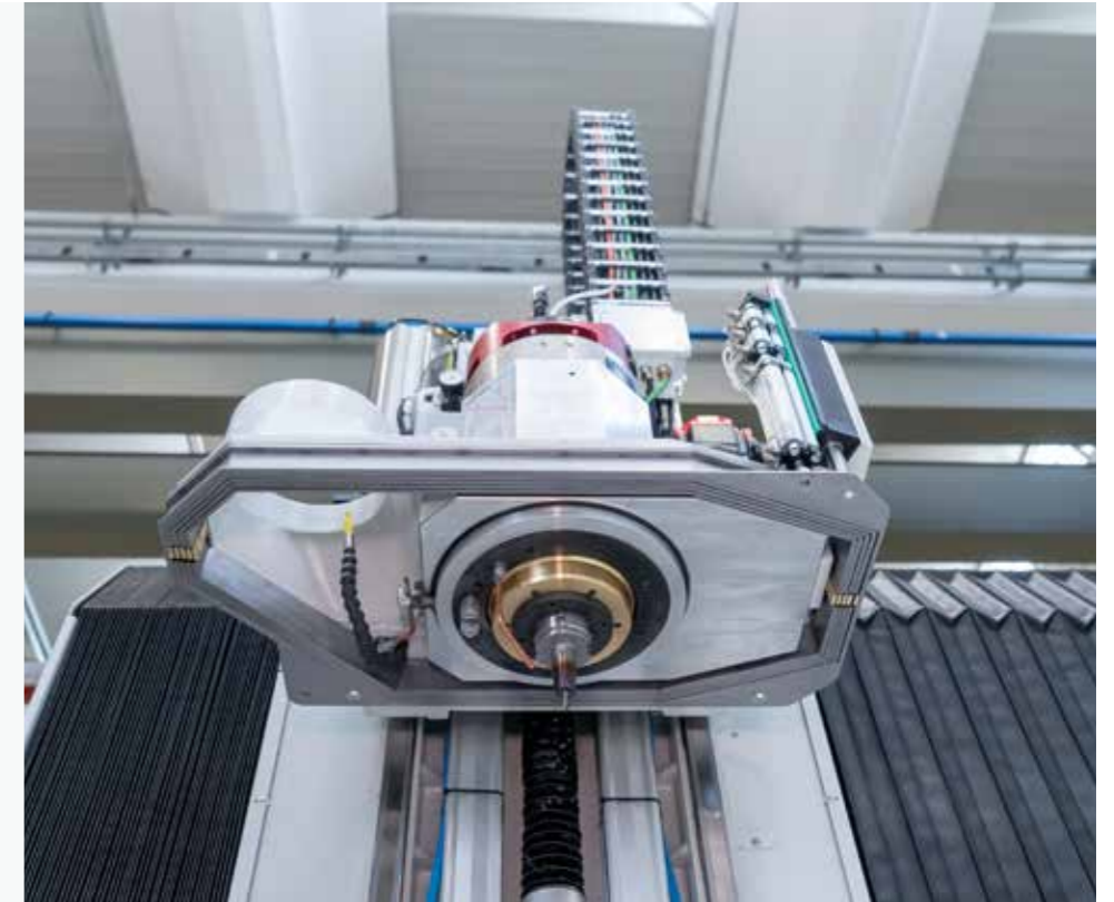
PX3 - KX3 Machining units for 3 or 4-axis configurations, with 12 to 32 kW spindles at 24,000 rpm.
