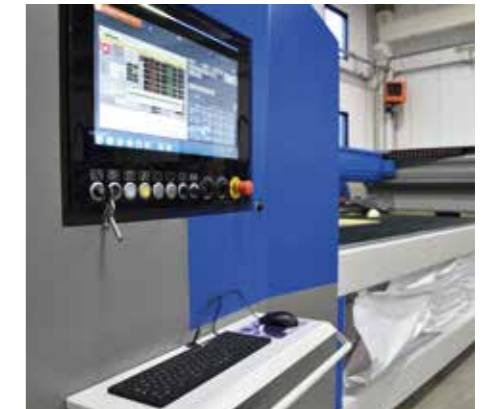
21.5" industrial PC Panel on the machine with touch display and HMI CMS Active interface.
