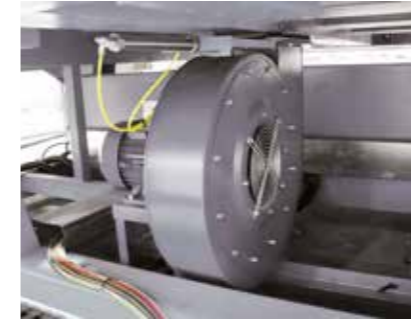
The work table is equipped with an air cushion which can be set in two positions, depending on glass dimensions and thickness
