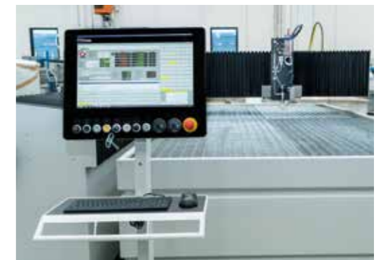
21,5" touch screen control panel on mobile trolley.
