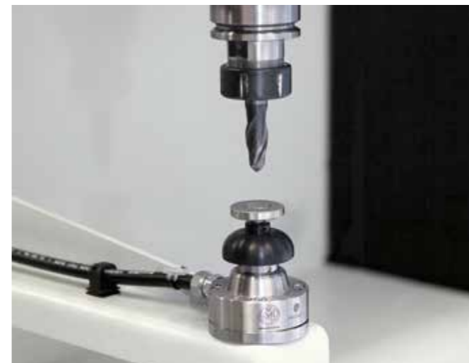
Contact sensor for checking and restoring rotary axes
