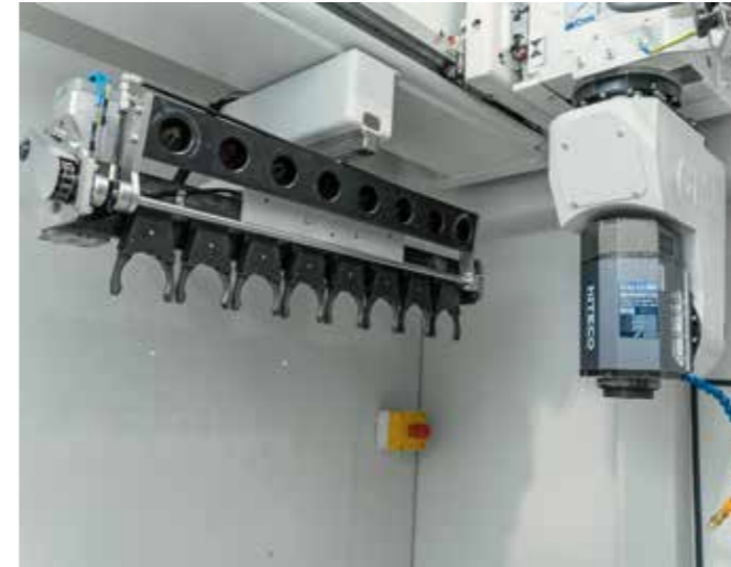
8-station tool storage that allows tools with a significant weight to be handled while simultaneously providing pressurized protection to the tool holder
