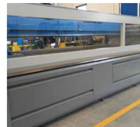
Front and rear safety doors with pneumatic movement to protect the cutting area and reduce the dispersion of water and abrasive material.
