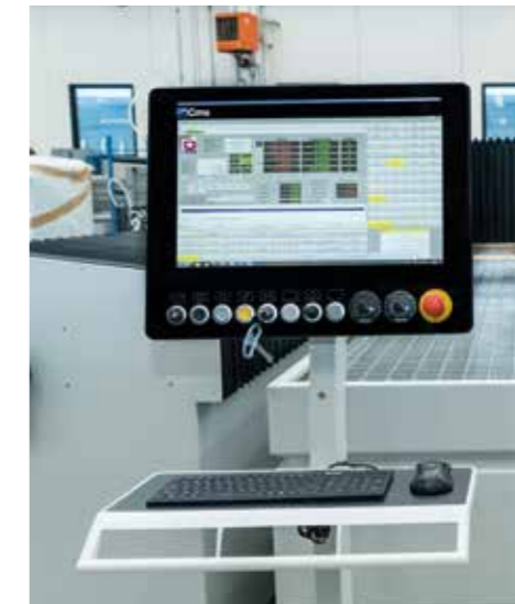
Console on a mobile trolley with 21.5" touch screen.
