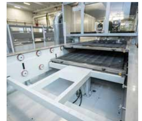
AUTOMATIC PALLET CHANGE Separate loading and unloading areas with automatic pallet movement via servomotor.
