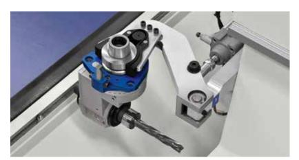
One position "Pick-up" tool changer with pneumatic positioning fitted on the mobile cross beam.
