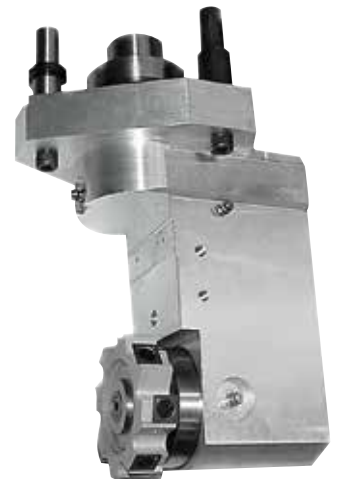
Head for cleaning 90° internal angles
