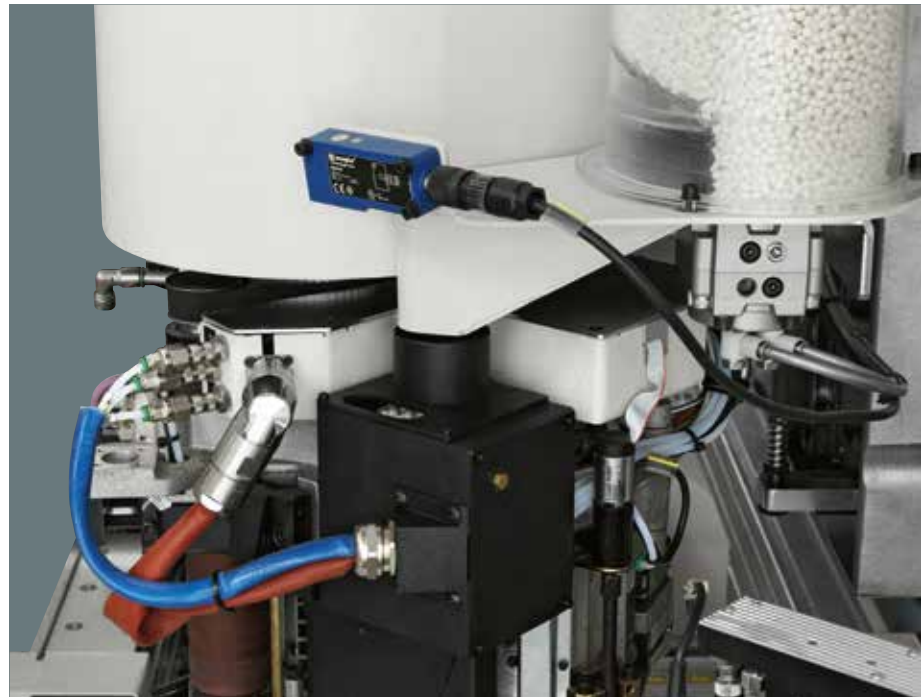
Glue is loaded in masked times into the granule feed system.
