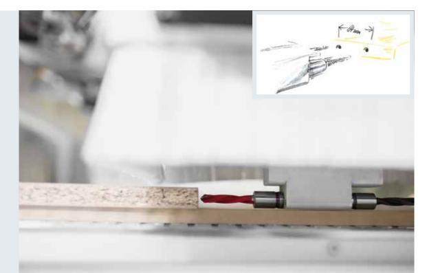
Ability to execute horizontal drilling with no need to lift workpieces from the spoilboard, due to lowered horizontal drilling heads.
