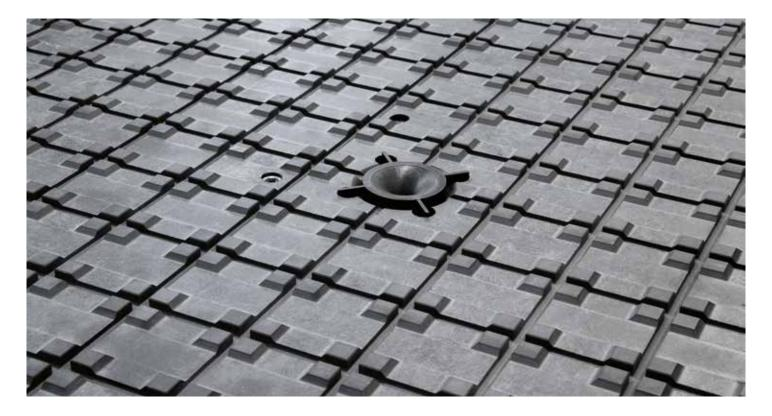
Any machining without removing the supporting panel and no obstacles due to the tubeless **X-POD pods**.
