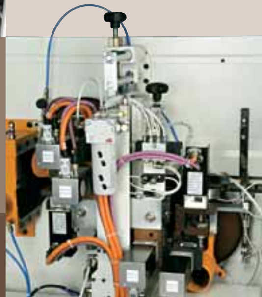
Multifunctional edgescraping unit
