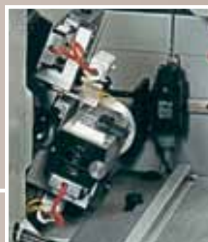
Multifunctional 4 motors corner rounding unit
