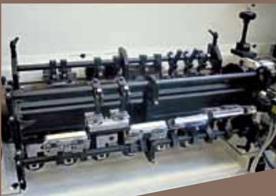
Pressure sectors exchange by revolver
