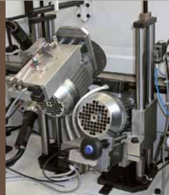
Buffing unit for aluminium edge
