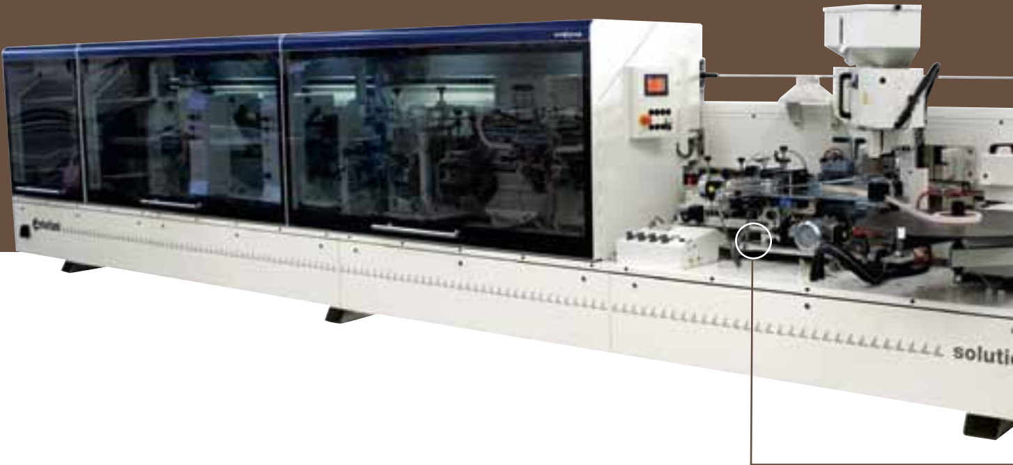
Thin, ABS and solid wood edges processing
