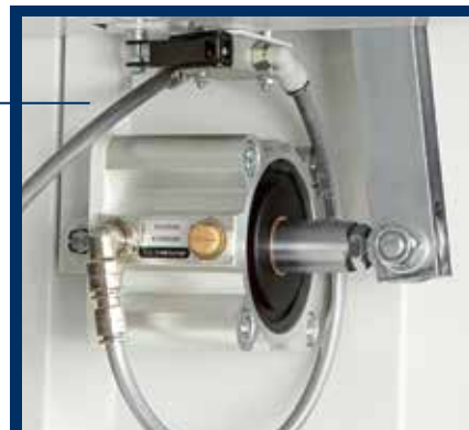
Automatic feed belt centering for a longer lifespan of the belt.
