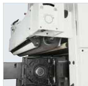
Buffing and structuring units on the outfeed of the working table for exclusive surface finishes.
