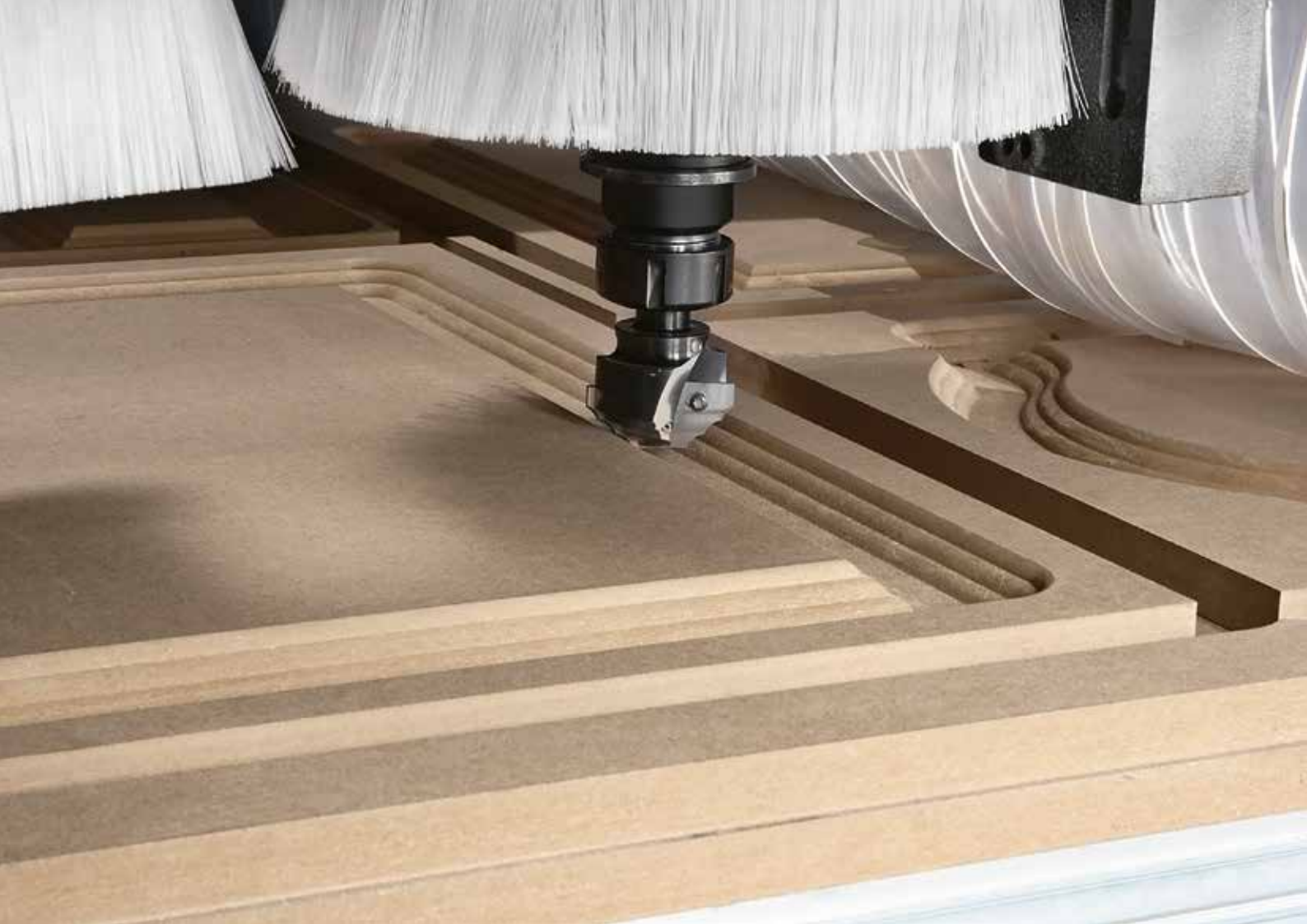
Optimal machining precision with the 3-axis electrospindle up to 24.000 rpm.
