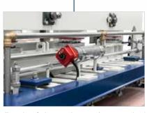
**Two electric heat exchangers** for pressurised air heating, powered by electricity to improve gluing quality.
