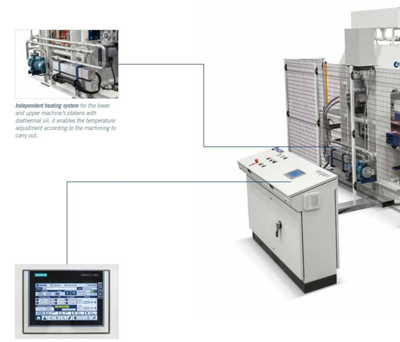
**Control panel with Siemens colour touch screen** The control panel is equipped with software that allows the total management of the press and to control machine's parameters in each working cycle phase.
