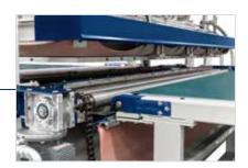
High efficiency with the double membrane pressing system The double membrane allows the two sides of the panel to be machined simultaneously, increasing productivity and working over several shifts.
